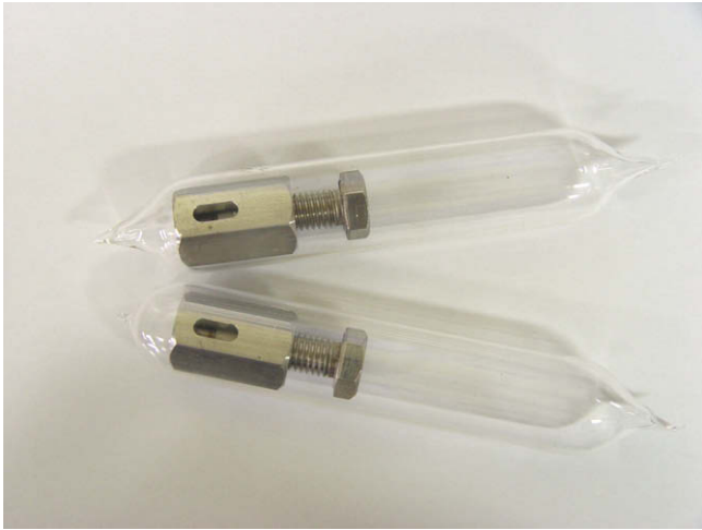
Fig. 1. A photo showing vacuum-sealed stainless steel clamps containing a diffusion couple of U–Zr–X and FMS.
